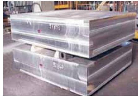
6 Sides milled with Lifting hole
