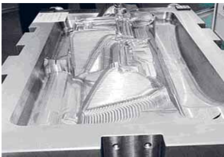
3D pre-Milled Dash board Mold
