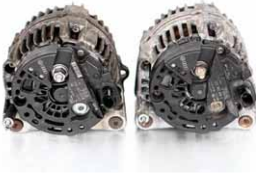
Product variance – two generators with different part numbers are visually identical.
