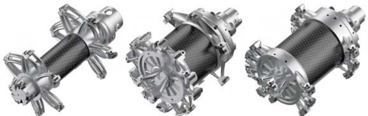
■ First-generation design (9.5kg) on the left, and latest tool design variants (less than 8kg) on the right for hassle free tool changing.
