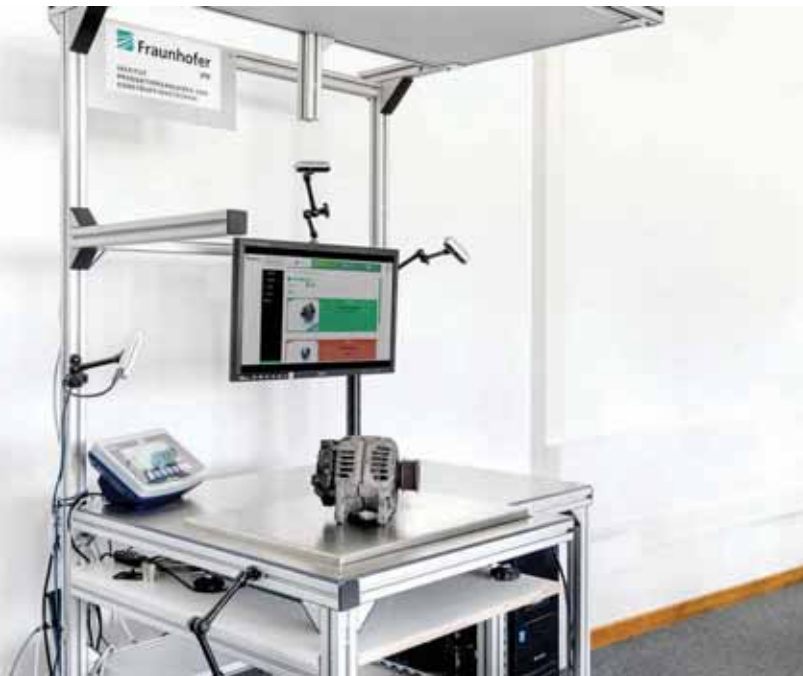
AI-supported assistance system for semi-automated sorting of used components.
