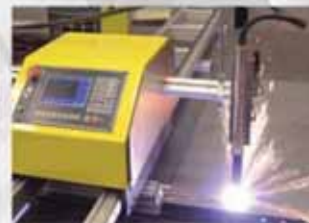
CNC PLASMA / OXYFUEL PROFILE GAS CUTTING UPTO 600MM THICKNESS
