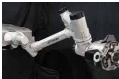
A robotic arm developed by Toyota for a vehicle called "Lunar Cruiser" to explore the lunar surface. TOYOTA MOTOR CORP. VIA AP
