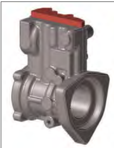
Fig. 1: Pump housing CAD model – gating at top
