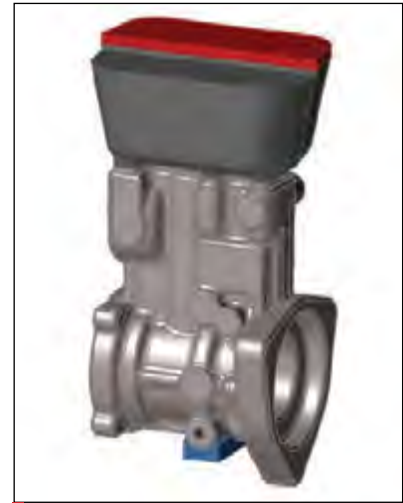
Fig. 6: Shot model including chillers
