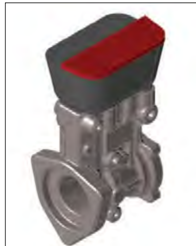
Fig. 3: Shot model with ingate
