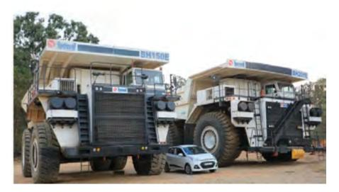
These trucks have eco-friendly emissions certificate engines with electronic fuel management system to deliver maximum power. Its wide body design, higher value metric capacity and low body weight ensures high stability and productivity. A state-ofthe-art AC drive system have been engineered to provide exceptional road performance with reduced maintenance.
