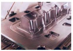
3D Machining to CAD Data
