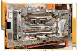
Injection molding tool for the Bumper
