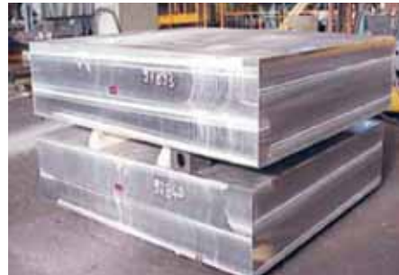
6 Sides milled with Lifting hole
