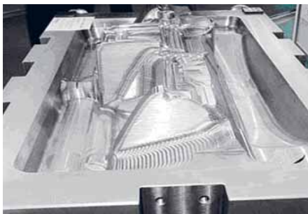
3D pre-Milled Dash board Mold
