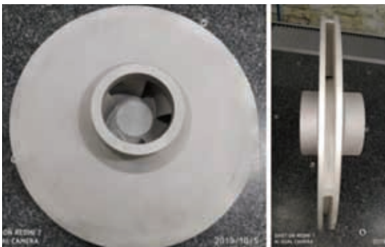
Figure 5 – Over 300mm size impeller 3D printed (replacement of investment casting process).
