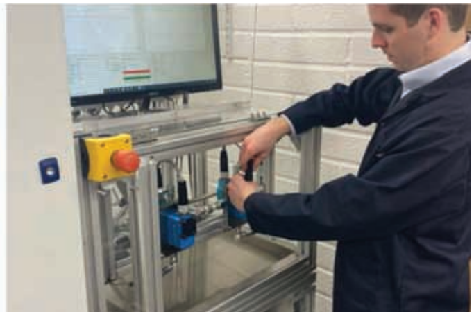
Testing an AM direct drive valve.
