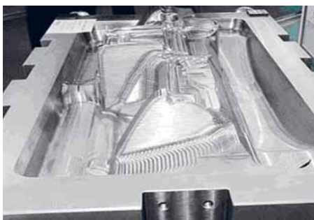
3D pre-Milled Dash board Mold
