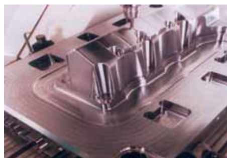
3D Machining to CAD Data
