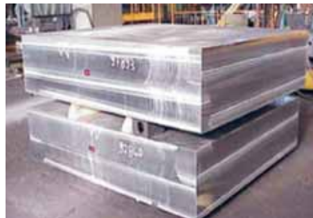
6 Sides milled with Lifting hole
