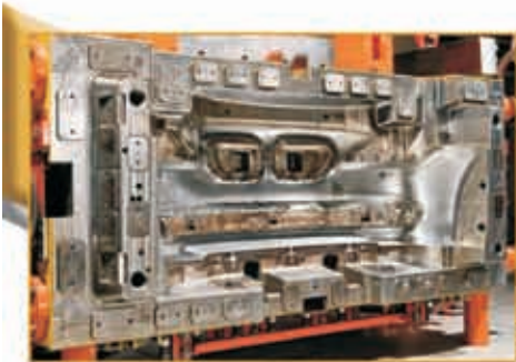
Injection molding tool for the Bumper
