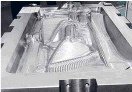
3D pre-Milled Dash board Mold
