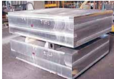
6 Sides milled with Lifting hole
