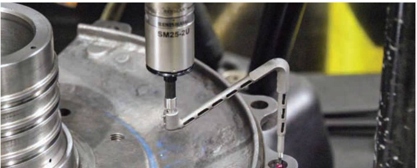
■ Custom stylus metal 3D printed on a RenAM 500Q system
