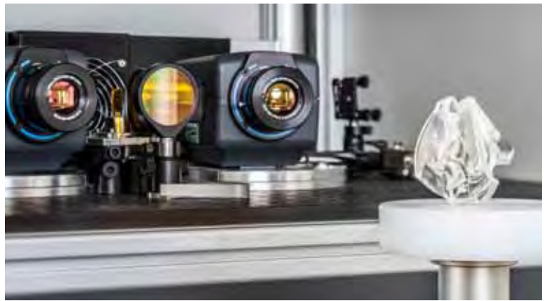
The system works with thermal radiation for the 3D detection of transparent objects.
