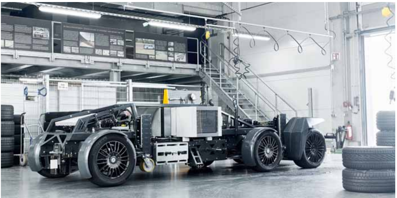
AVA enables precise monitoring of the friction characteristics of tires during braking maneuvers on dry and wet roads.
