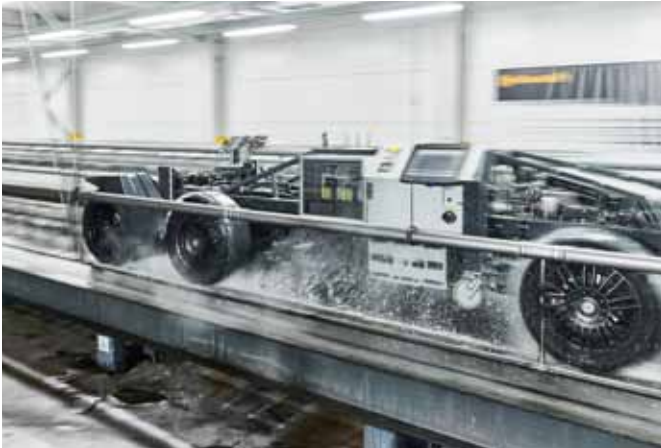
With the AVA, Continental combines the advantages of a model-independent test method with the controlled and reproducible test environment.
