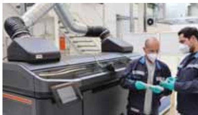
Two Volkswagen employees check the quality of structural parts produced using the binder jetting process for car production in front of the prototype of the special printer at the high-tech 3D printing center in Wolfsburg.
