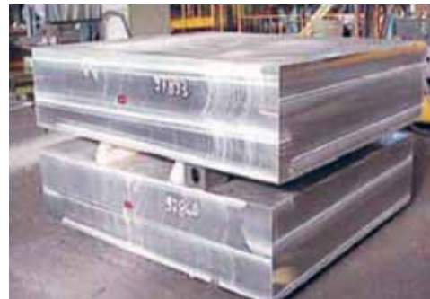
6 Sides milled with Lifting hole
