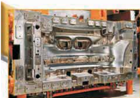
Injection molding tool for the Bumper
