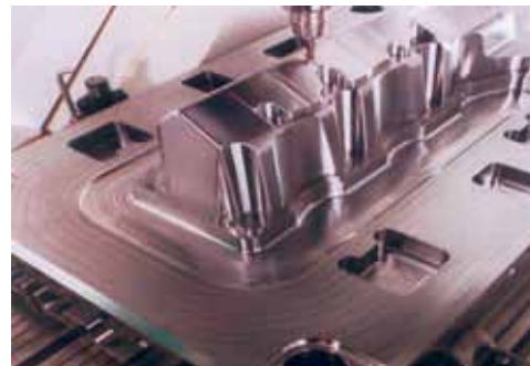
3D Machining to CAD Data
