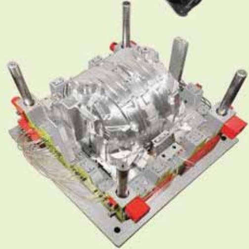
Mould: Protector-Front Fender Mould tonnage: 2500T
