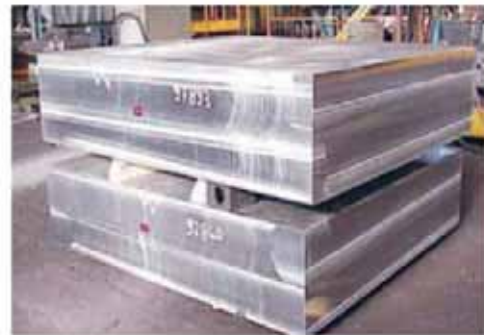
6 Sides milled with Lifting hole
