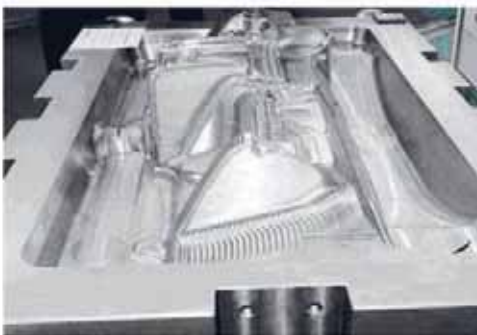
3D pre-Milled Dash board Mold
