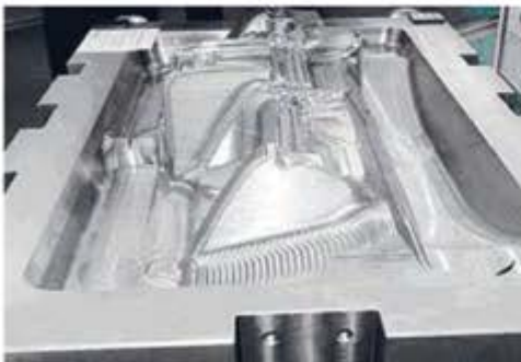
3D pre-Milled Dash board Mold
