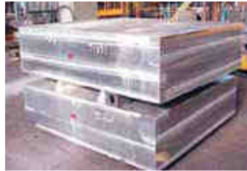
6 Sides milled with Lifting hole
