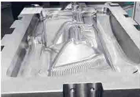
3D pre-Milled Dash board Mold
