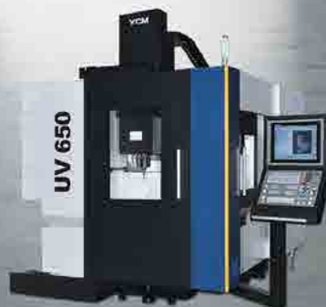
UV650 High Performance 5-Axis Vertical Machining Center
