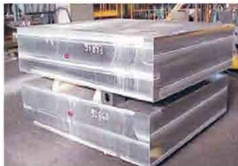
6 Sides milled with Lifting hole
