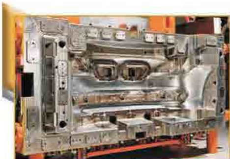
Injection molding tool for the Bumper
