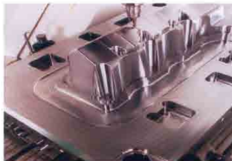
3D Machining to CAD Data
