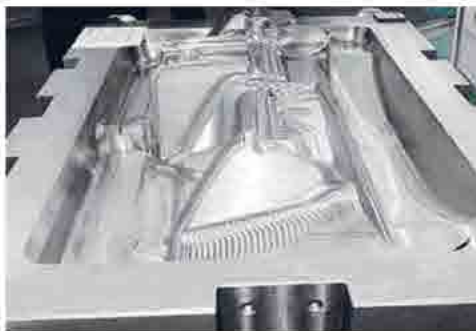
3D pre-Milled Dash board Mold
