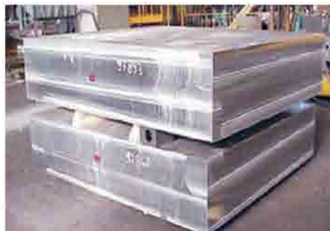
6 Sides milled with Lifting hole
