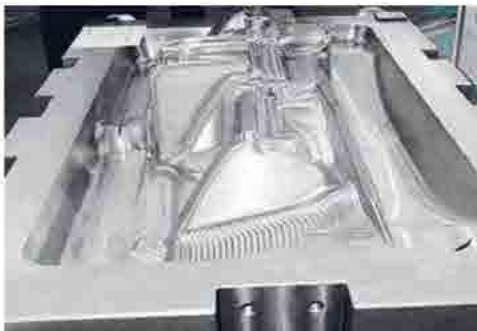
3D pre-Milled Dash board Mold
