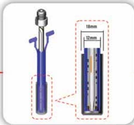
MICRO NOZZLE WITH COOLING
