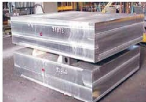
6 Sides milled with Lifting hole
