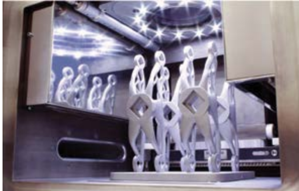
Figure 4: Bleu car hinge component in RenAM 500M build chamber.
