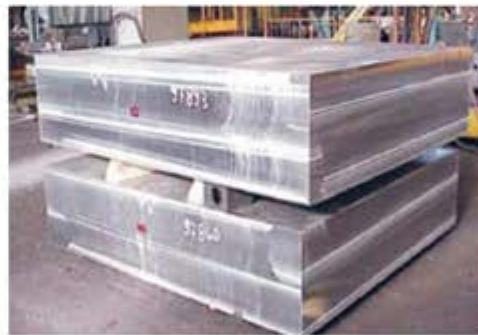
6 Sides milled with Lifting hole
