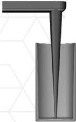
3PLATE MOLD WITH COLD RUNNER
