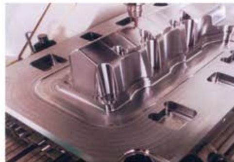
3D Machining to CAD Data
