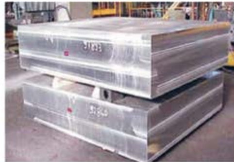
6 Sides milled with Lifting hole
