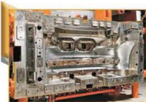
Injection molding tool for the Bumper
