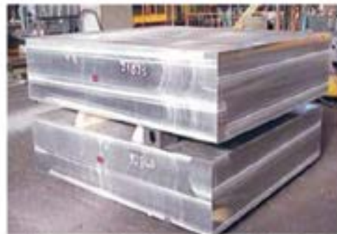
6 Sides milled with Lifting hole
