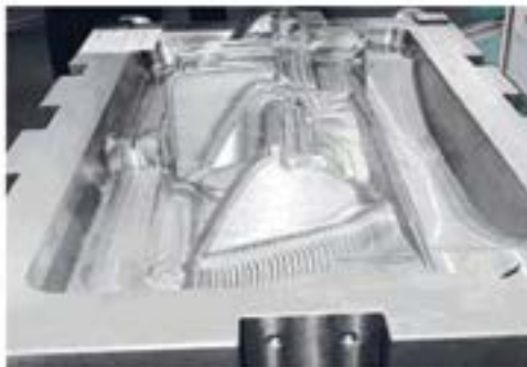
3D pre-Milled Dash board Mold
